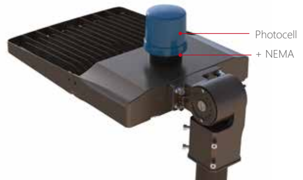
NEMA+Photocell 3-PIN: Lighting Switch 5-PIN: Expandable DALI or 0-10V Dimming 7-PIN: Expandable DALI and 0-10V Dimming
